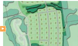
Conventional Layout: Seek to maximize number of lots, but increase length of paved surfaces, utilities and storm water infrastructure
