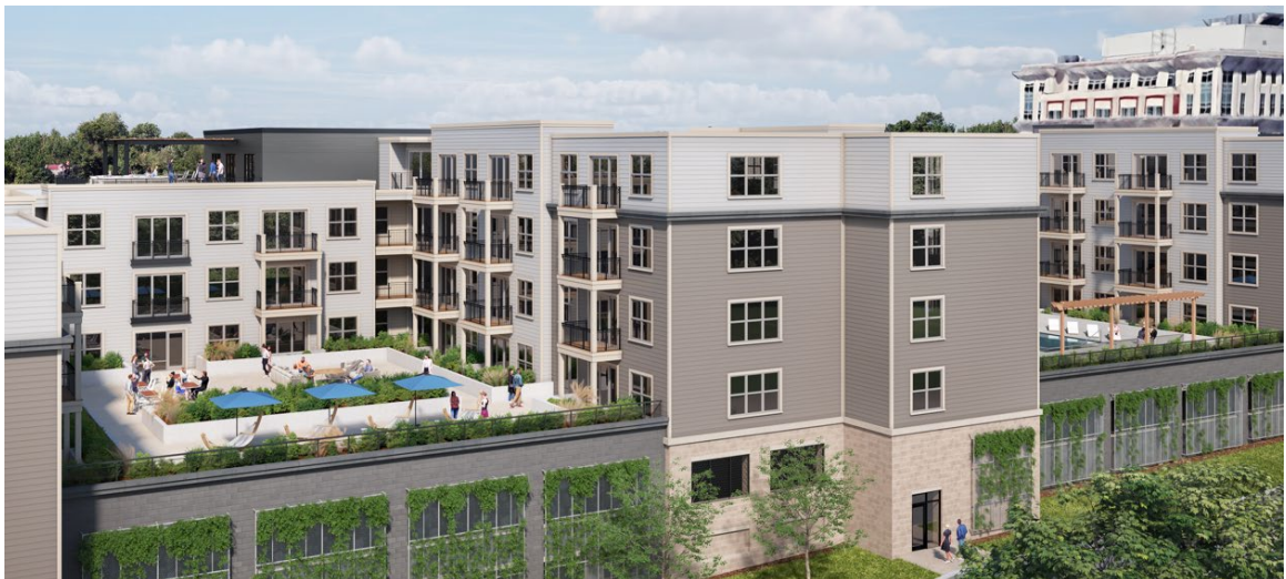
Figure 12: A rendering of the Wollerton Alley façade showing the solar-oriented recesses (amenity courtyards) used to tame the massing.
